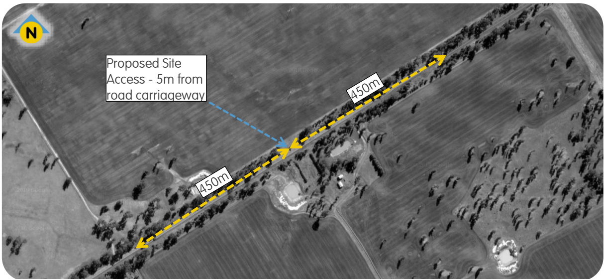
Figure 10 Sight Distance Assessment - Proposed Site Access
